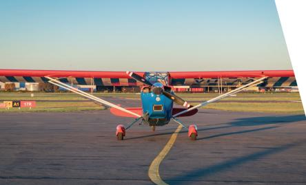
Lycoming AEIO-360-H1B Analogue Avionics with Dials + EFIS D10A Aerobatic Category MTOW: 816kgs Cruising Speed 120kts Aerobatic Rating +6/-5G 2 Seater (Tandem)
