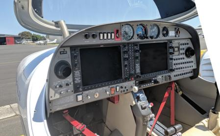
Continental CD-135 Engine x 2 FADEC single lever power controls Garmin G1000 Avionics Maximum Take-Off Weight (MTOW) 2000kgs Cruising Speed 150kts @ 60% Power 4 Seater
