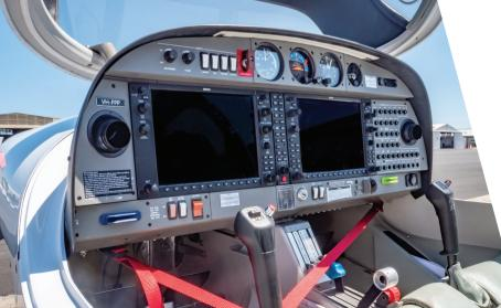
Continental CD-135 Engine/Lycoming IO-360 Garmin G500 or Garmin G1000 Avionics Maximum Take-Off Weight (MTOW) 1150/1200kgs Cruising Speed 130kts 4 Seater
