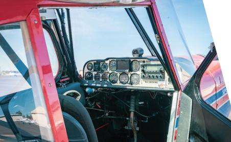
Lycoming AEIO-360-H1B Analogue Avionics with Dials + EFIS D10A MTOW: 886kgs Cruising Speed 120kts Conventional (Tailwheel) Undercarriage 2 Seater (Tandem)
